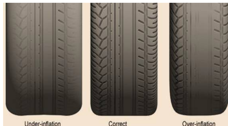
Figure (b). Tyre wear patterns observed for different tyre inflation pressures
